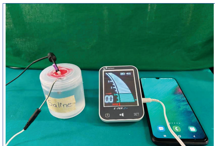
[Table/Fig-4]: Smartphone in close proximity to Electronic Apex Locator (EAL) without any mode activation (Group 2).
